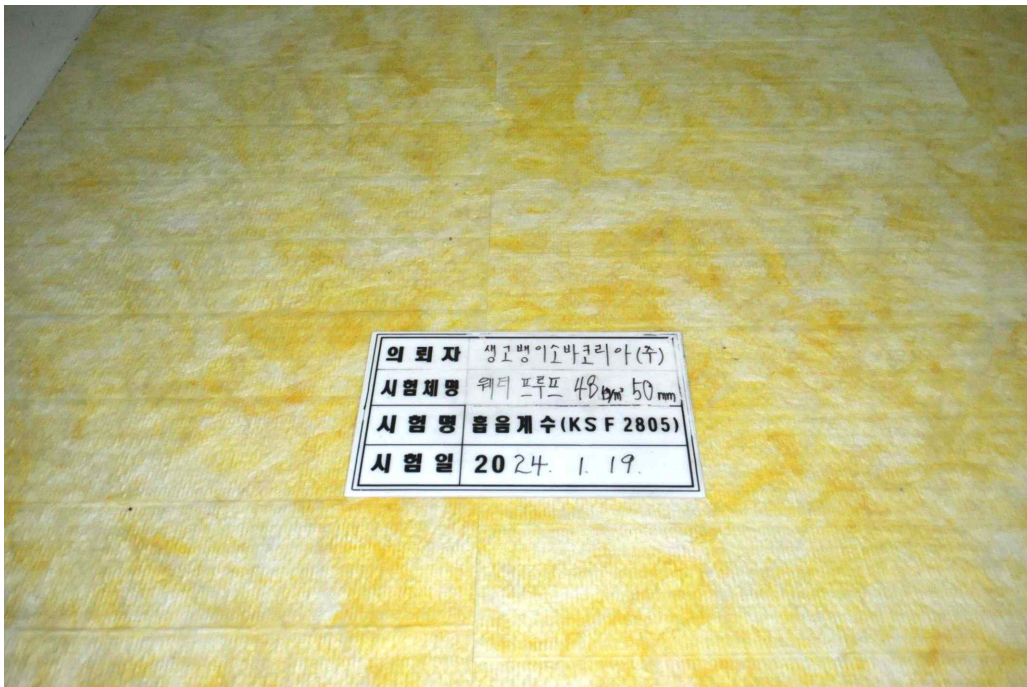
[PHOTO 1] Test specimen arranged in reverberation room
