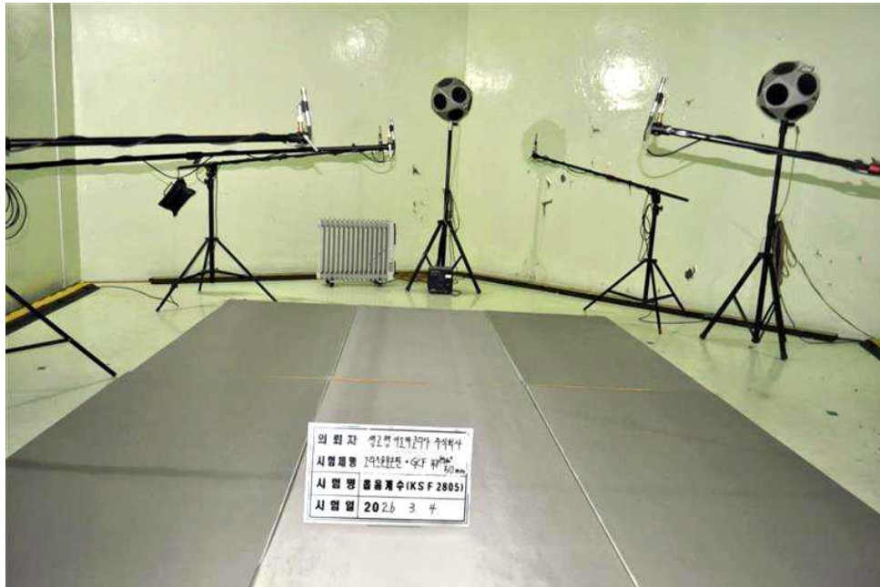
[PHOTO 1] Test specimen arranged in reverberation room
