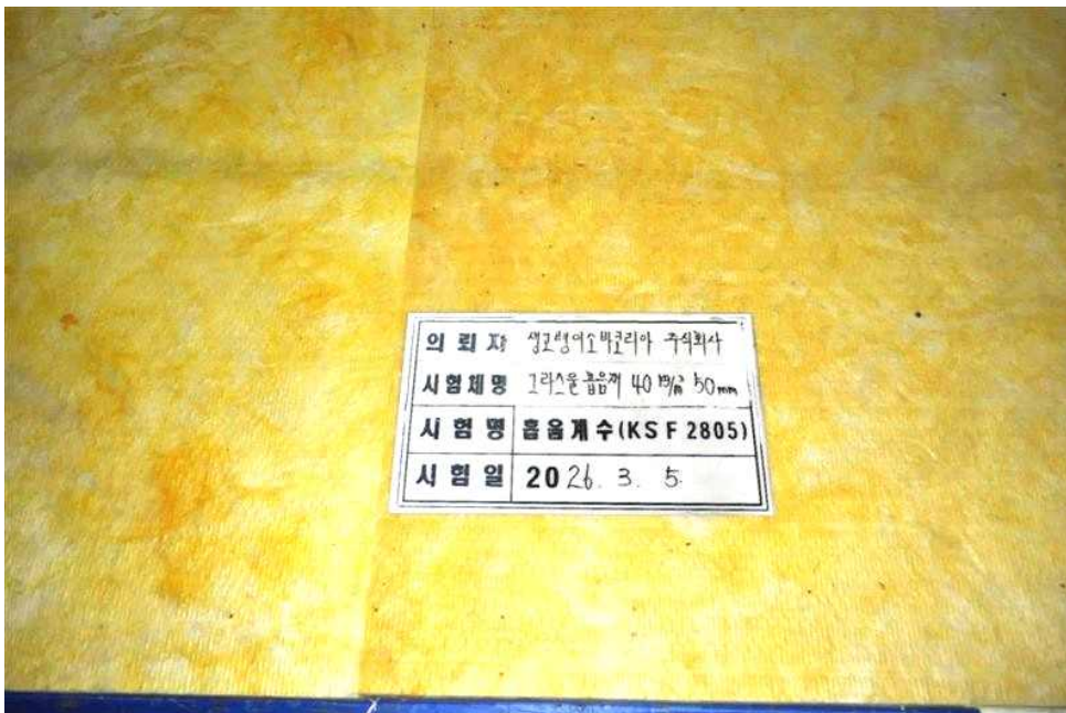
[PHOTO 2] Details of the test specimen arrangement
