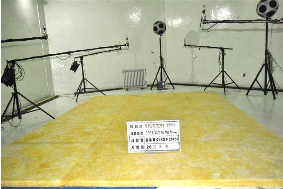
[PHOTO 1] Test specimen arranged in reverberation room
