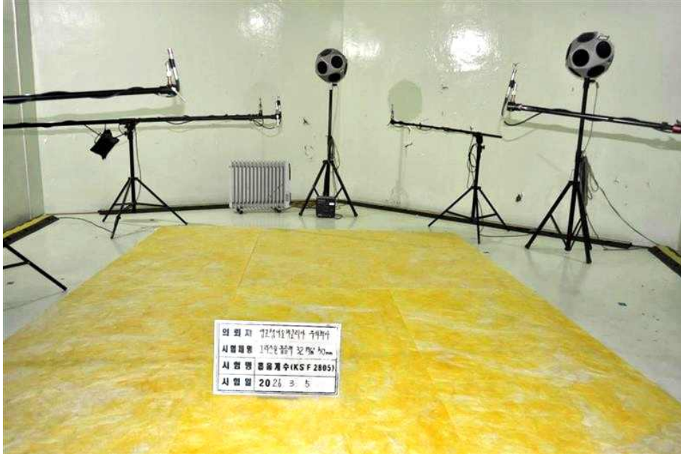
[PHOTO 1] Test specimen arranged in reverberation room
