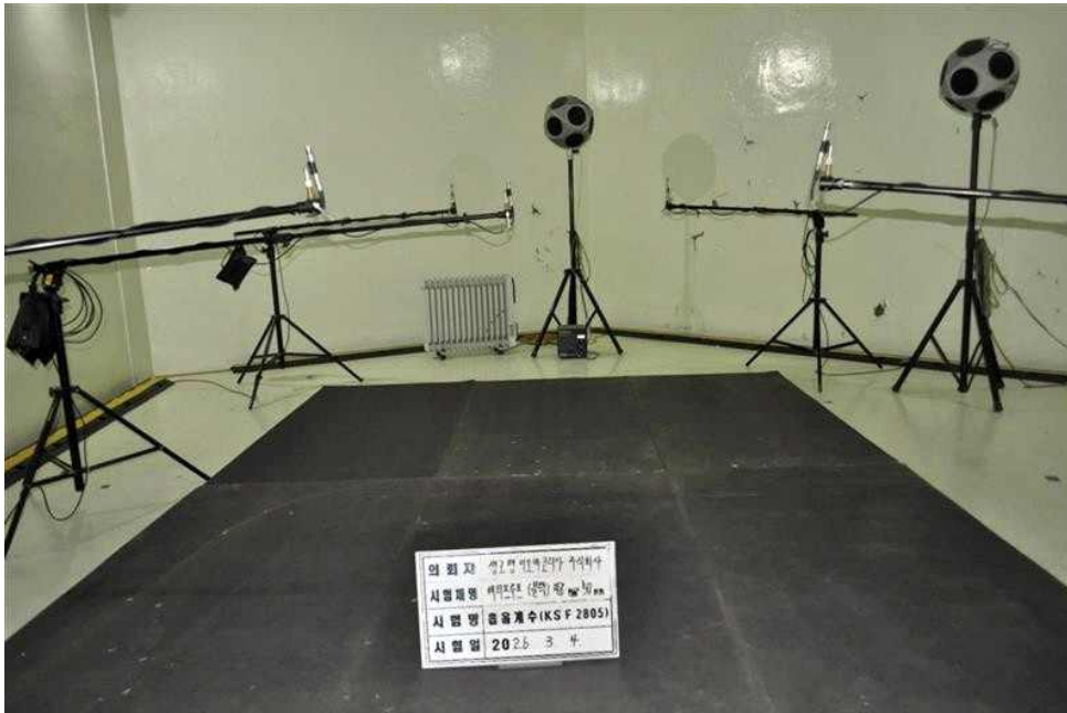
[PHOTO 1] Test specimen arranged in reverberation room
