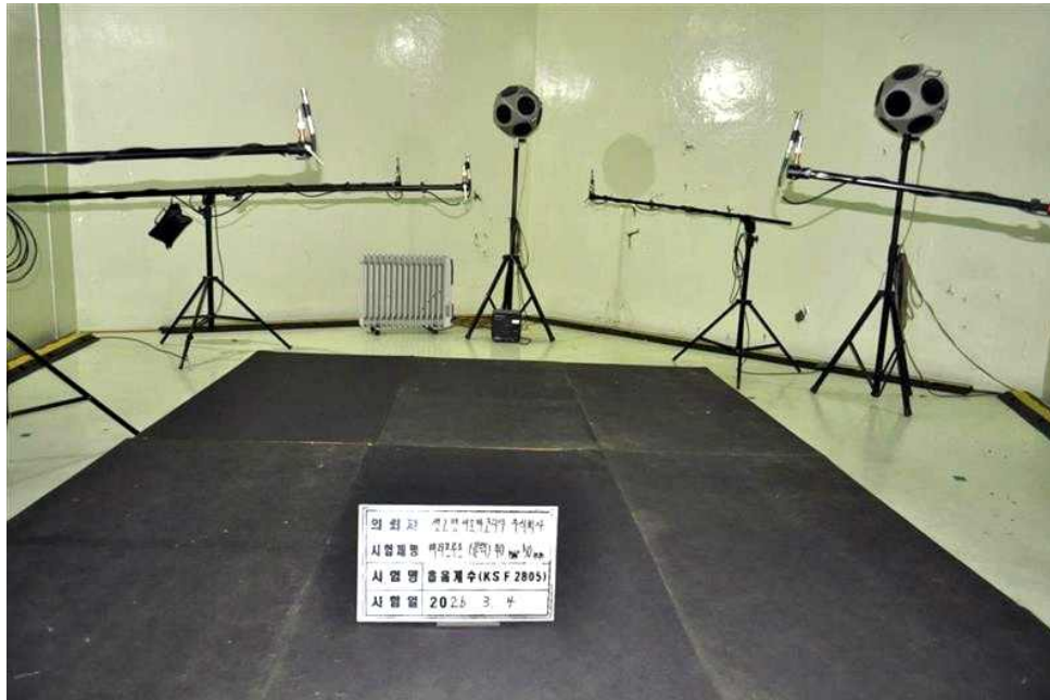
[PHOTO 1] Test specimen arranged in reverberation room
