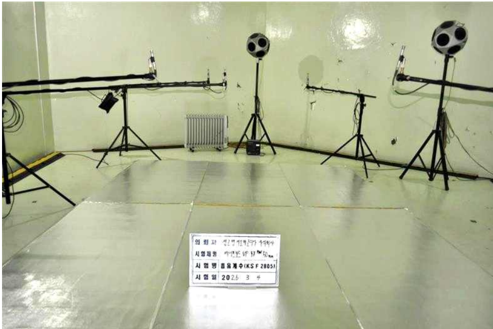
[PHOTO 1] Test specimen arranged in reverberation room
