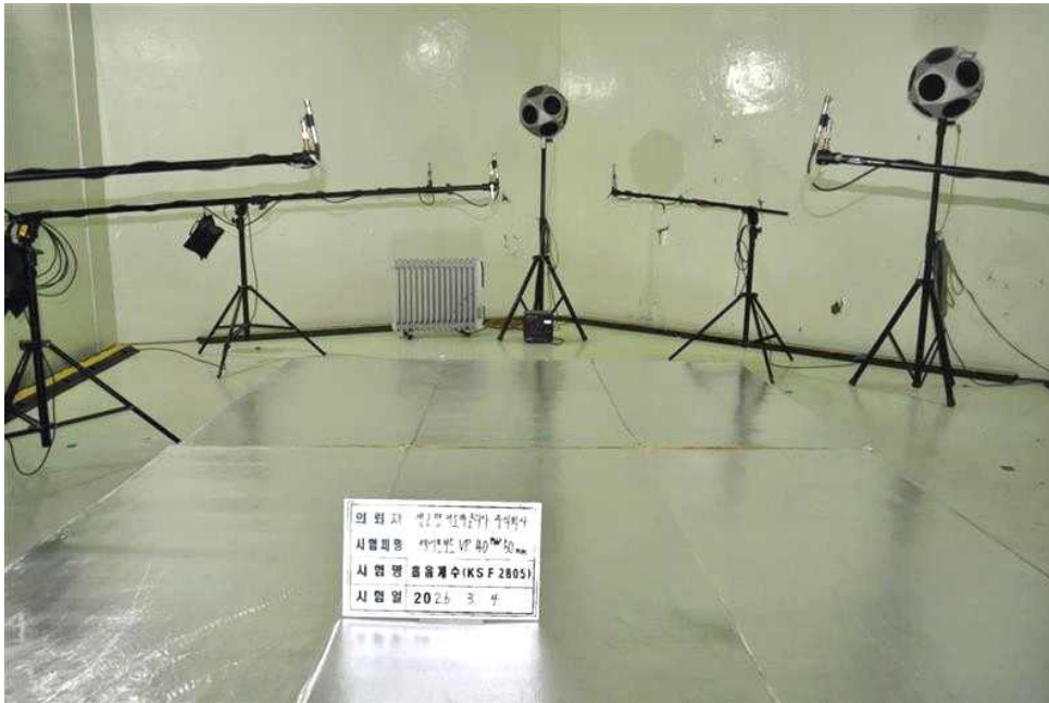
[PHOTO 1] Test specimen arranged in reverberation room
