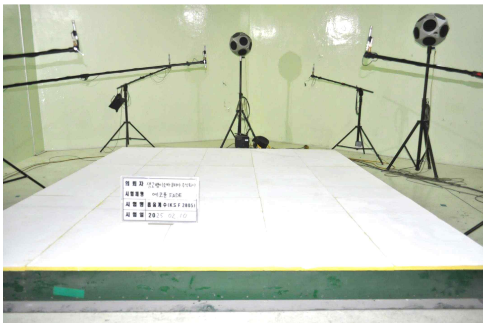
[PHOTO 1] Test specimen arranged in reverberation room
