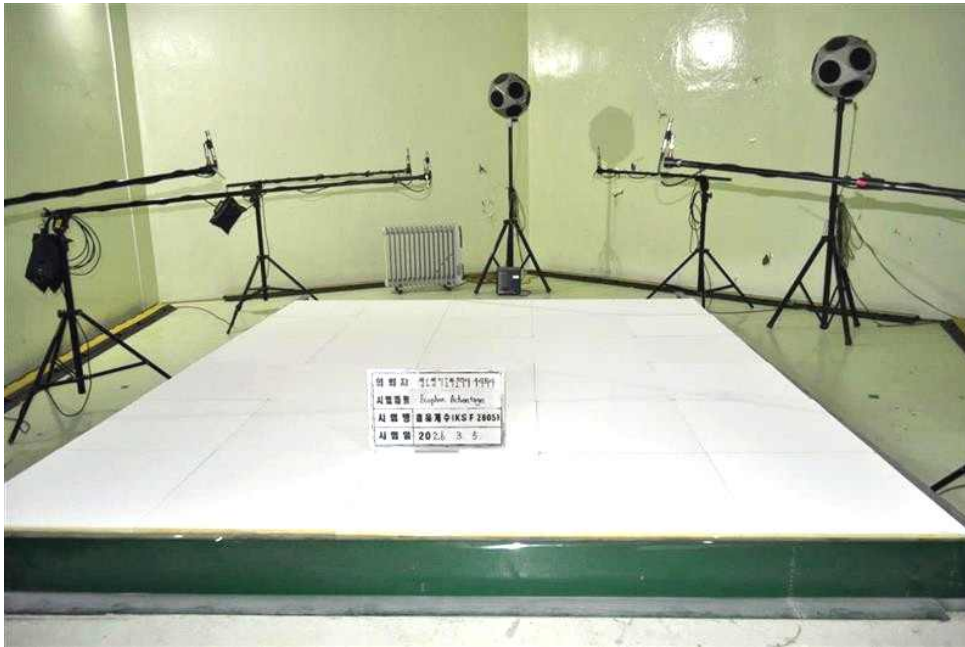
[PHOTO 1] Test specimen arranged in reverberation room
