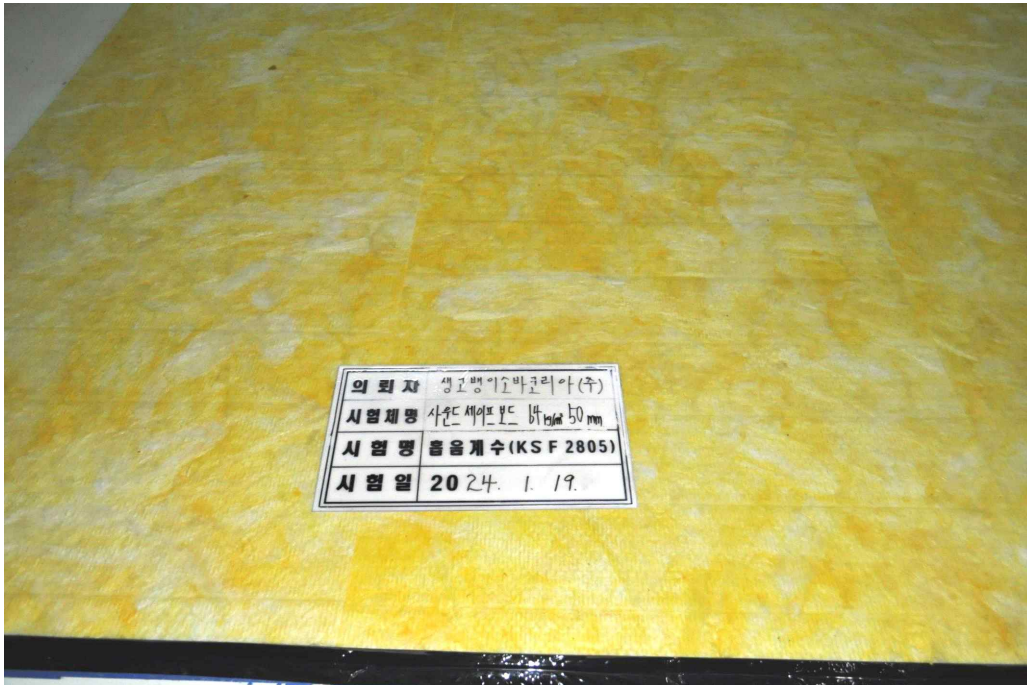
[PHOTO 1] Test specimen arranged in reverberation room
