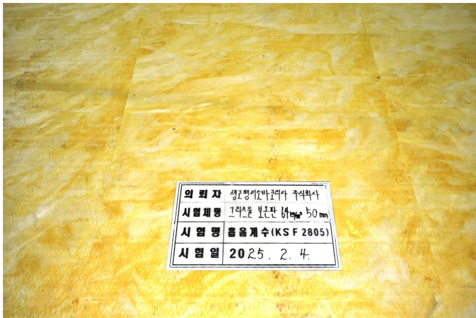
[PHOTO 2] Details of the test specimen arrangement
