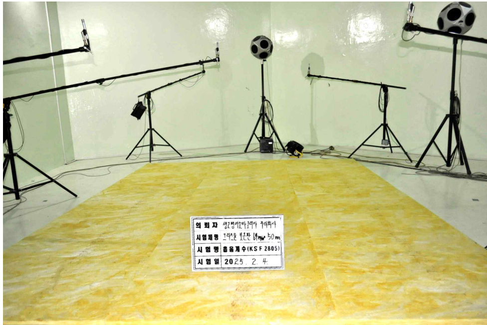
[PHOTO 1] Test specimen arranged in reverberation room
