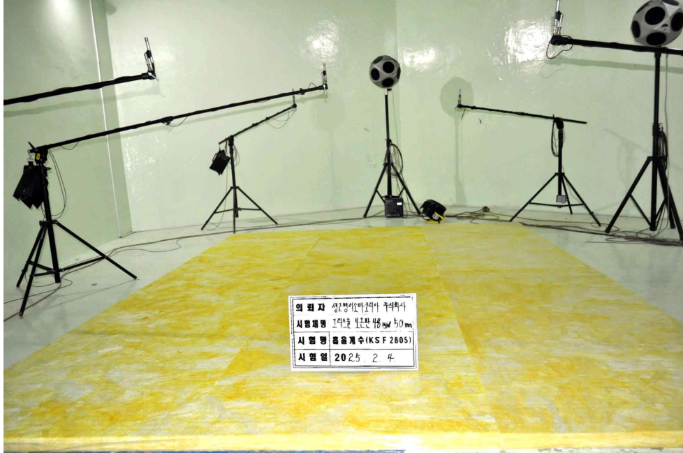
[PHOTO 1] Test specimen arranged in reverberation room
