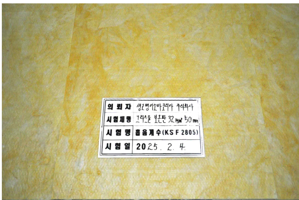
[PHOTO 2] Details of the test specimen arrangement
