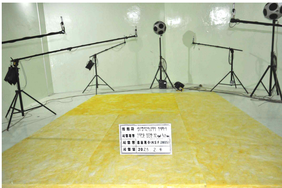
[PHOTO 1] Test specimen arranged in reverberation room
