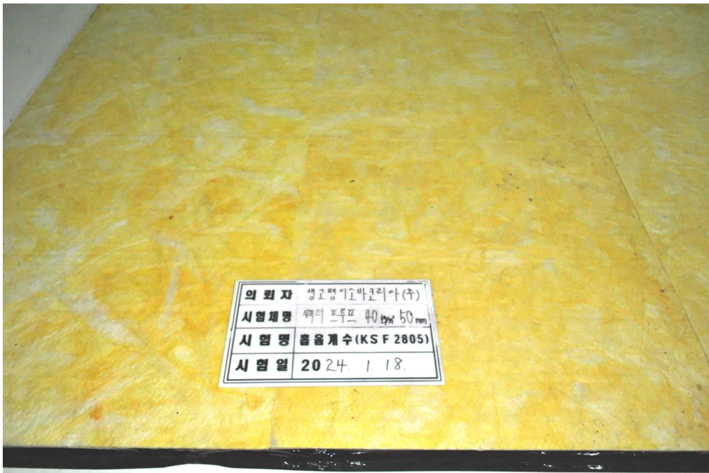
[PHOTO 1] Test specimen arranged in reverberation room
